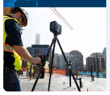
Set up the FARO Focus Premium Laser Scanner at the determined position. This can be accomplished manually or by driving the scanner via the Flatness Check<sup>™</sup> App on iOS tablets, preferably a LiDARenabled tablet. (\*Note: Flatness Check<sup>™</sup> App still works with other iOS tablets) Select the appropriate resolution depending on the device's distance from the slab and perform the scan.
