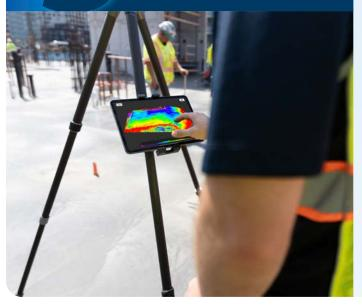
Scans are immediately transferred into the app where one or multiple scans can be analyzed. The app then takes the user through the required steps with results that can be visualized using the iPad's AR capabilities and overlaying to reality. The process takes 5 to 15 minutes depending on slab size and number of scans.
